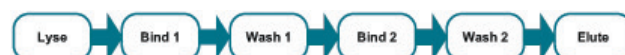
Figure 3: sbeadex unique technology includes a two step binding mechanism enables users a second wash step using pure water. This results in higher yields, higher DNA purity and efficiently removes all inhibiting salts and alcohols. As no alcohol is used, drying and evaporation of the DNA is not necessary resulting in a time, money and waste minimising extraction,
